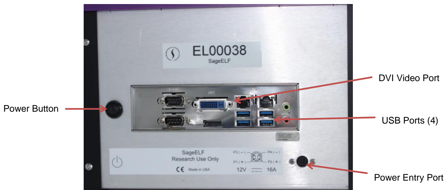
Figure 3.2. Rear Panel of the Sage ELF
