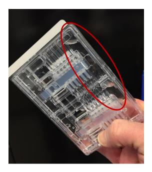
Aggregate and collect air bubbles in the upper buffer chambers
