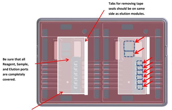
Seal tape by pressing firmly on the edges of the ports.
