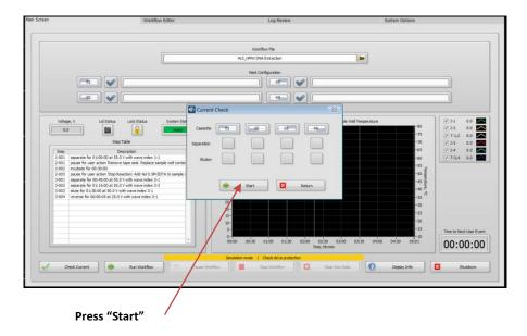
3. The routine will first test the separation electrodes, then test the elution electrodes, and complete within a few minutes. After a successful test, all boxes will fill with green check marks. Press "Return" to continue
