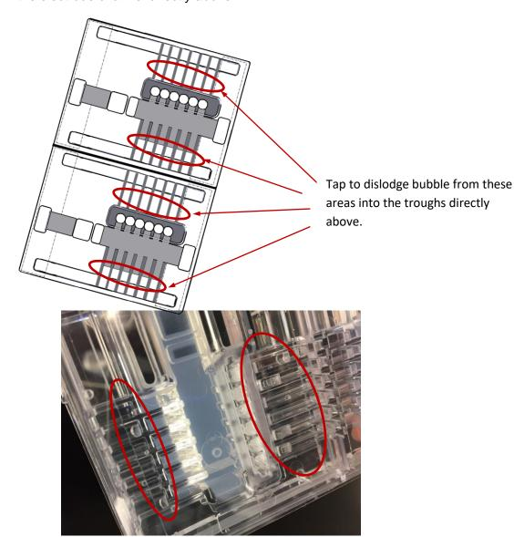
Bubbles in the elution paths can interfere with collection
