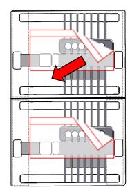
3. Using a wide-bore pipette tip, remove the contents of the elution modules.
