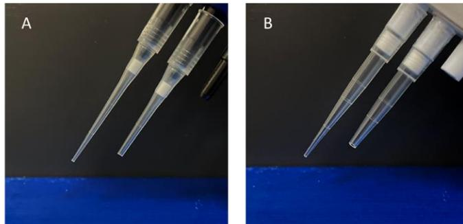
A. 20uL pipette tips (uncut and cut) B. 200uL pipette tips (uncut and cut)
