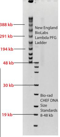
A gel image showing resolution of fragments from a gel run with the Pippin Pulse (Part No. PPI-0200) using the pre-set "5-430kb" protocol. The gel was run on a 12 X 14cm gel for 16 hours. The gel was cast with 0.75% Lonza SeaKem® GOLD agarose on the Sage Science midi gel box (Part No. PGB-1000) and 0.5X KBB buffer (Part No. KBB-1001).
