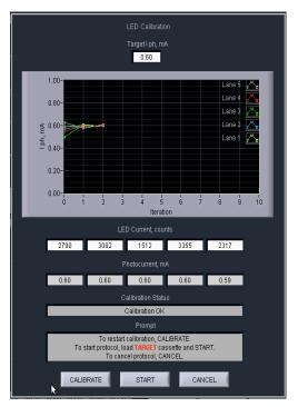
The Calibration sub-window after a successful calibration. If the status window reads "Calibration OK", proceed to the next step.
