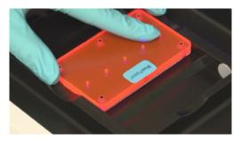
Correct placement of the calibration fixture.
