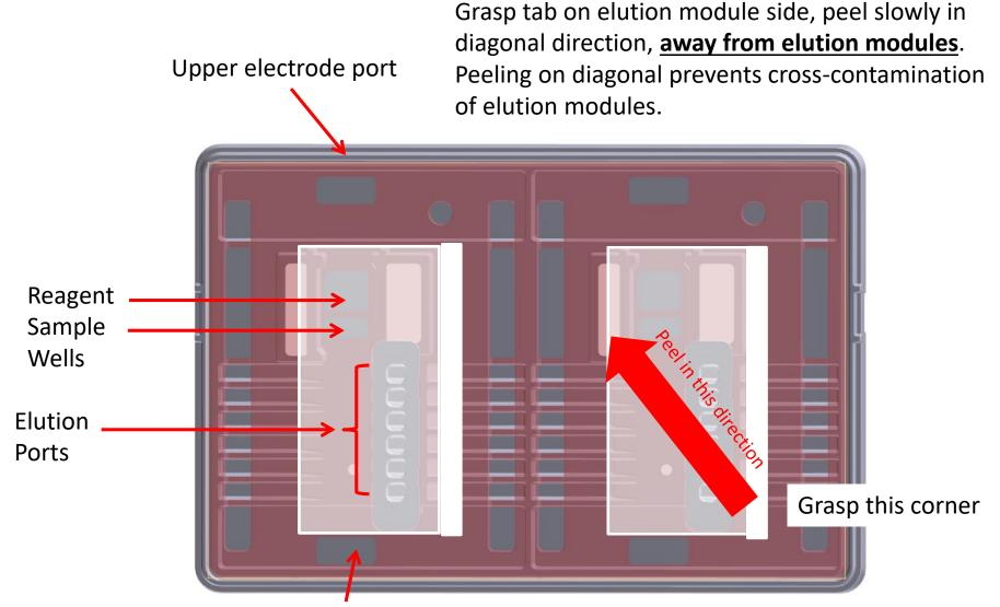
Lower electrode port, remove SDS-rich buffer here after Stage 1.
