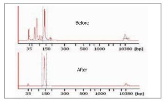
Using a PippinHT, unwanted artifacts can be removed from microRNA libraries using a range setting. 24 samples can be processed with a 30 minute run time.
