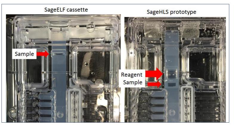
In the Sage HLS prototype, the gelembedded sample is cast in the sample well, while lysis reagents are loaded in reagent well. For fragmentation or transposasemediated library prep, the reagent well is emptied and refilled with nuclease or transposase reagents for the second electrophoresis step. Size fractionation and electroelution also takes place in the second electrophoresis step.
