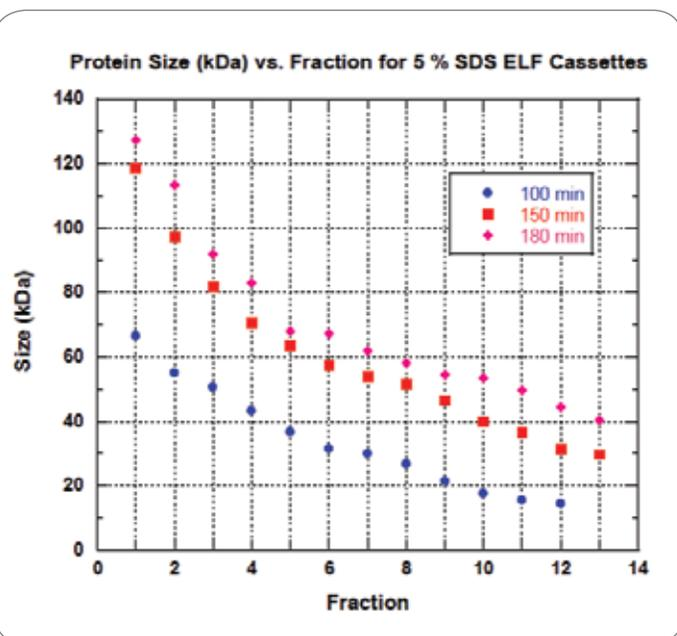
Fractionation ranges for a 5% agarose protein collections at three run times.
